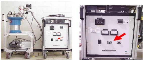
High temperature furnace (~1,600°C)
