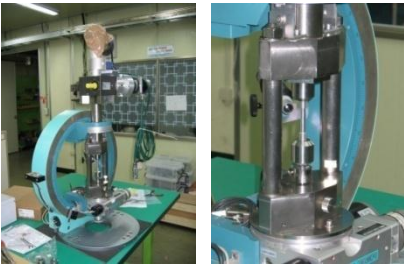
Loading device for Four Circle Diffractometer
