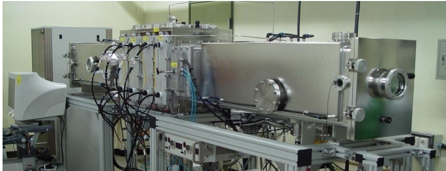
Large sputtering chamber for mirror coating of 1.2m length
